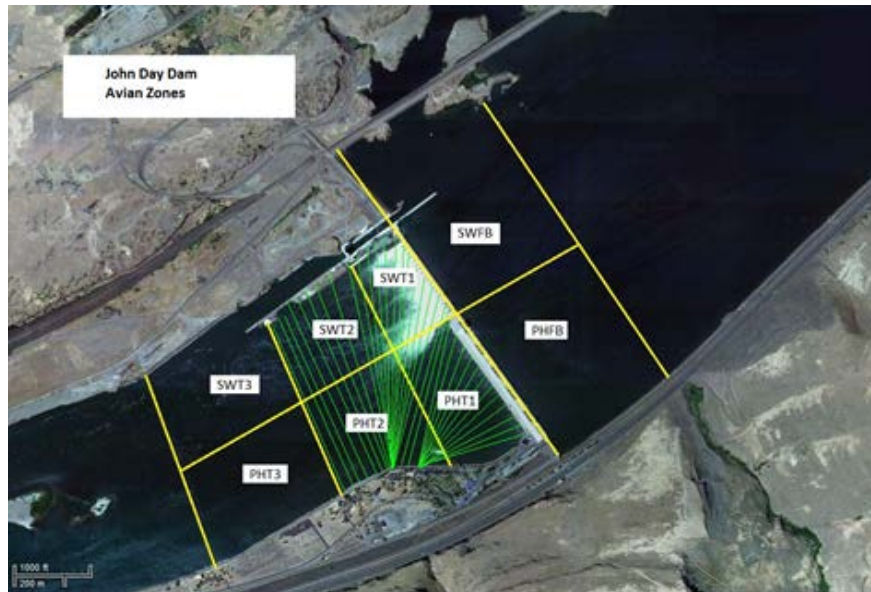
Figure 3: Avian array at JDA Tailrace BRZ installed in 2010 and re-tensioned for 2017 (Powerhouse Forebay-PHFB, Spillway Forebay-SWFB, Spillway Tailrace zones 1-3 [SWT1-SWT3], Powerhouse Tailrace zones 1-3 [PHT1-PHT3]).
